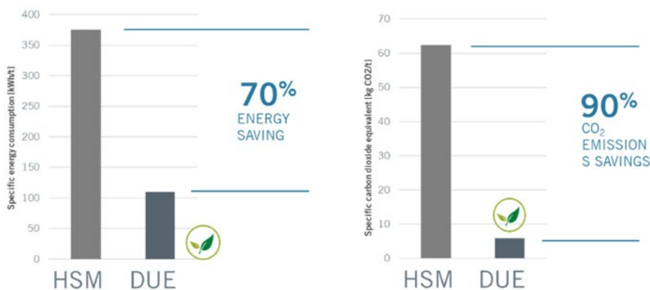
Fig.5 - Energy saving and CO 2 emissions reduction: comparison between conventional HSM and DUE.
