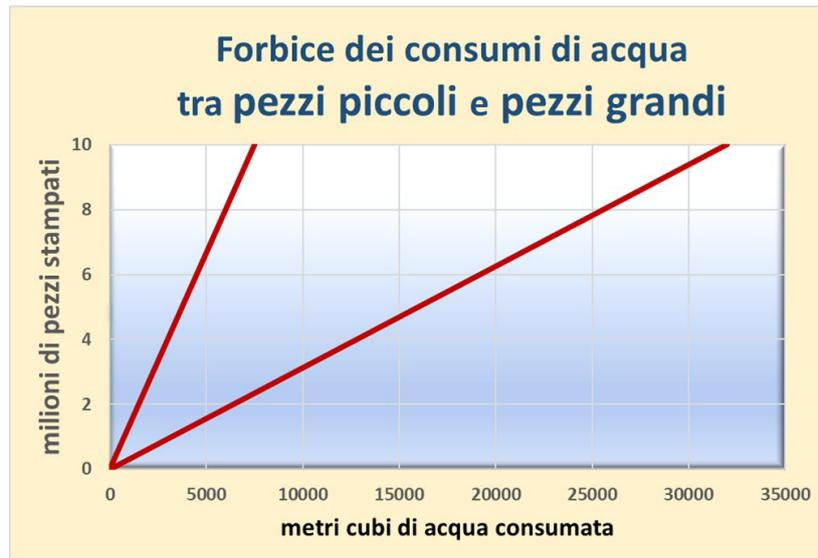
**Fig.2** - Consumo di acqua con i distaccanti base acqua [2] / *Water consumption with water-based release agents.*
