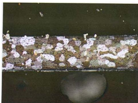
**Fig.5** - Dopo simulazione brasatura 600 °C x 1h - 100x / After brazing sim cycle at 600°C x 1 h – 100x
