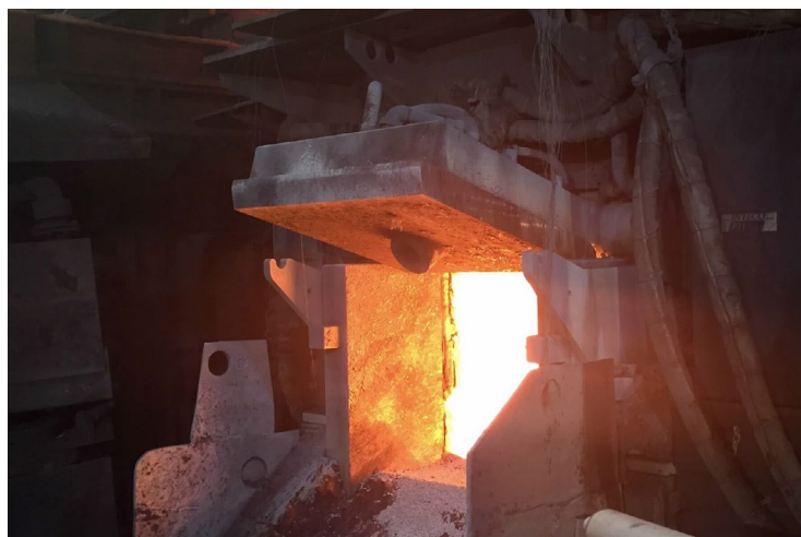
Fig.4 - SwingDoor™ in furnace inspection position.
