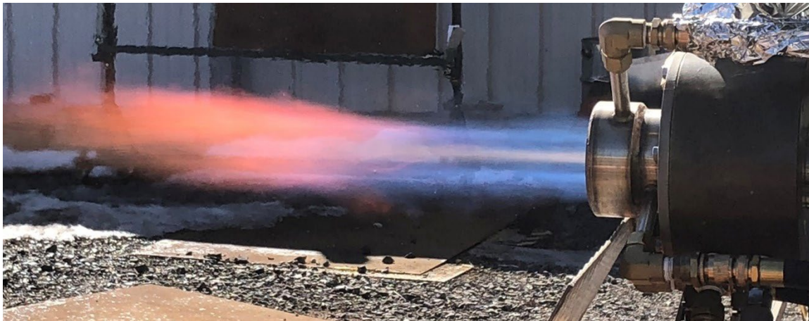
Fig.8 - Testing of 3-in1 Injector.
