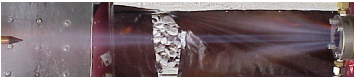
Fig.10 - Test with a CoJet in injection mode using 100% hydrogen as fuel.
