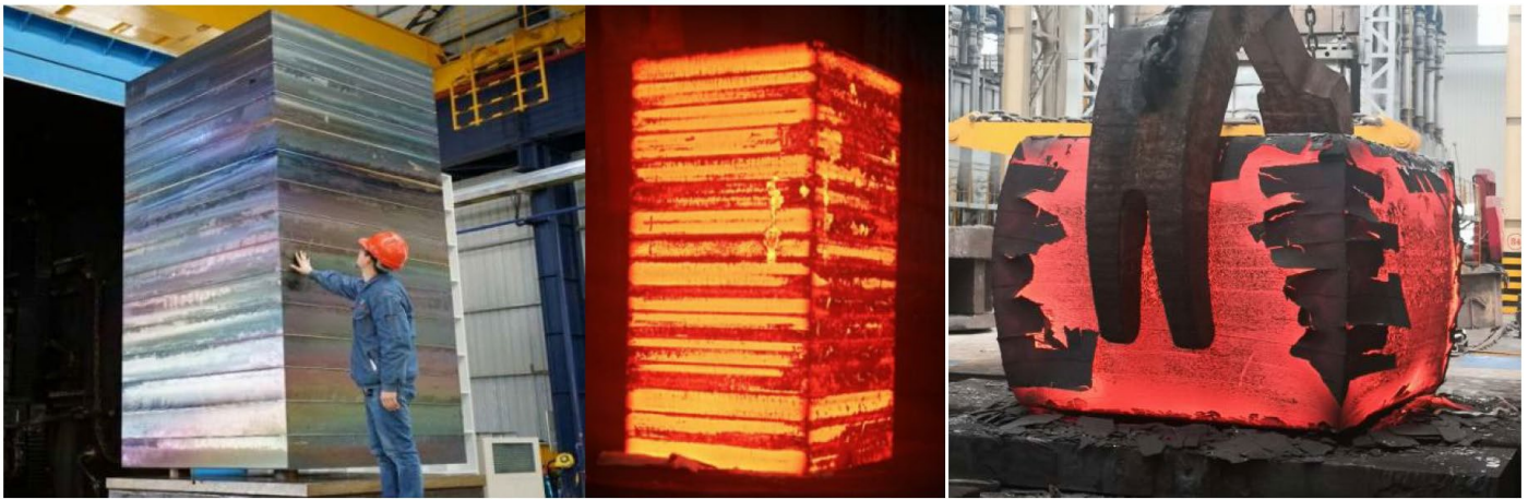
Fig.3 - Construction forming process of 316H steel slab.
