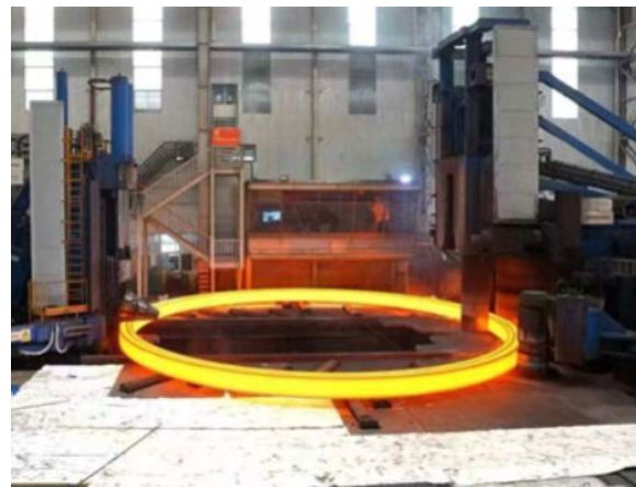
Fig.5 - Two steps rolling process of ring.
