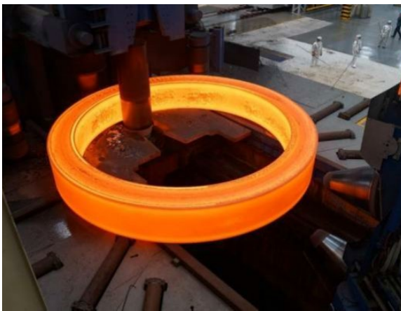
Fig.5 - Two steps rolling process of ring.
