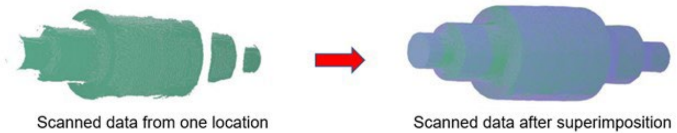
Fig.5 - Overlaying scanned data.
