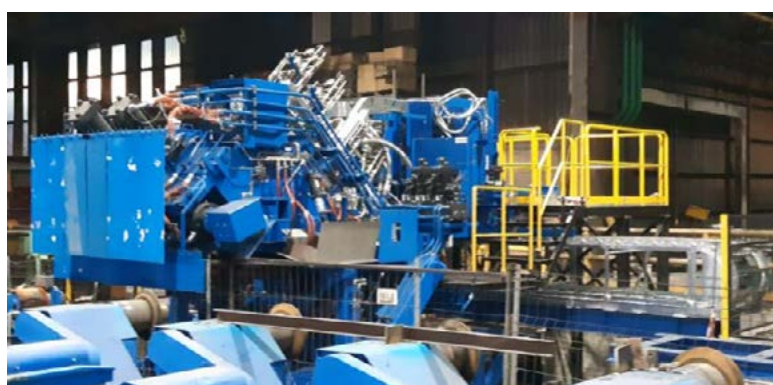
Fig.19 - Disposition billets welding machine.
