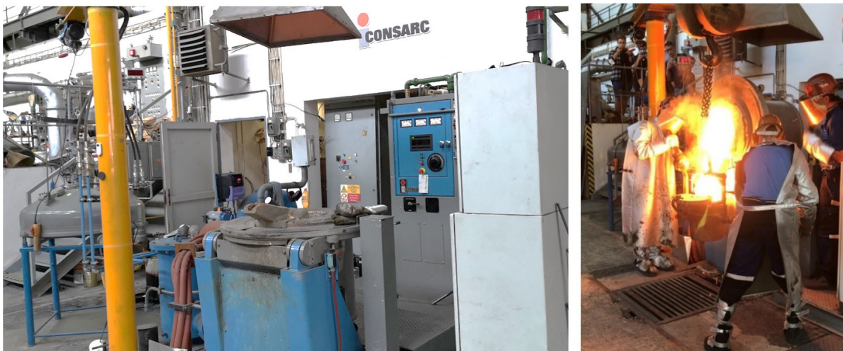
Fig.5 - Tapping stage of trial heat with 1.3243 tool steel at Brno University of Technology.[3]
