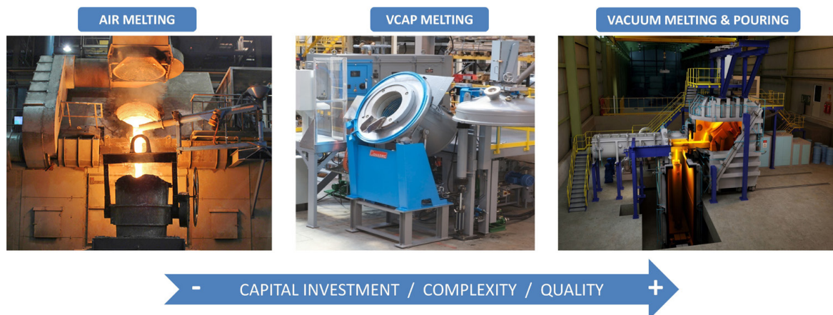
Fig.2 - Sketch of VCAP technology as a mixture of air melting and vacuum melting (VIM) technologies.
