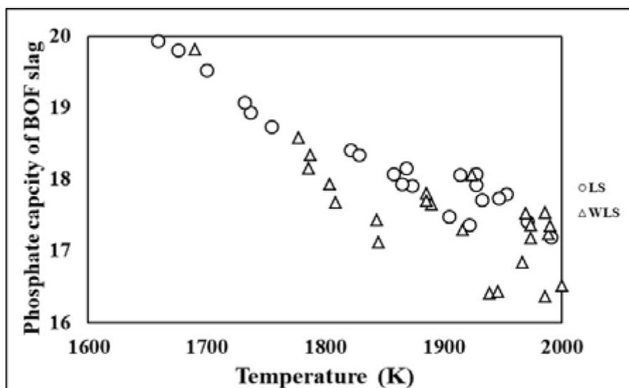
**Fig.10** -Variation of phosphate capacity of BOF slag as a function of temperature-with and without ladle slag addition.
