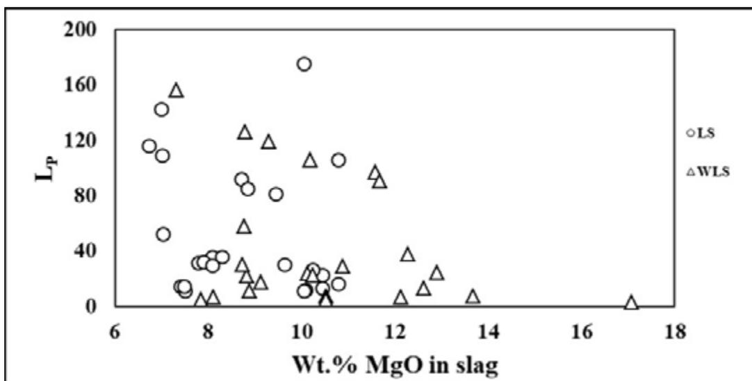
**Fig.9** - Variation of  $L_p$  as a function of wt. %MgO in BOF slag: with and without ladle slag addition.
