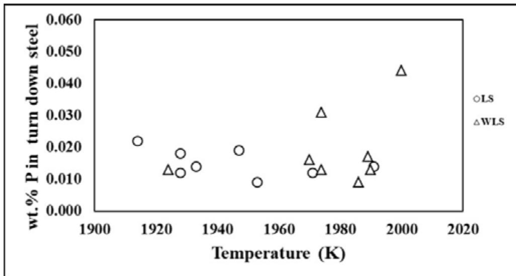
**Fig.8** - Turn down phosphorus content in steel as a function of temperature in BOF: with and without ladle slag addition.
