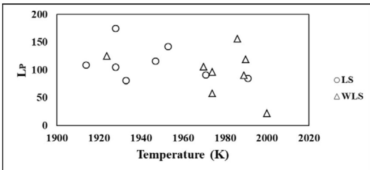
**Fig.7** -Variation of  $L_p$  as a function of opening temperature in BOF: with and without ladle slag addition.
