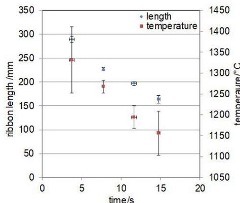
**Fig.4** - Ribbon length and temperature at impact in dependence on the transfer time between furnace and tipping of the crucible.
