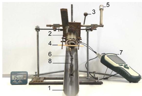
**Fig.1** - Inclined plane test in operation; consisting of 1) an inclined trough, 2) a crucible holder, 3) a trigger lever, 4) a re-taining device, 5) balancing weights, 6) a type-S thermocouple, 7) a datalogger and 8) slag ribbon.
