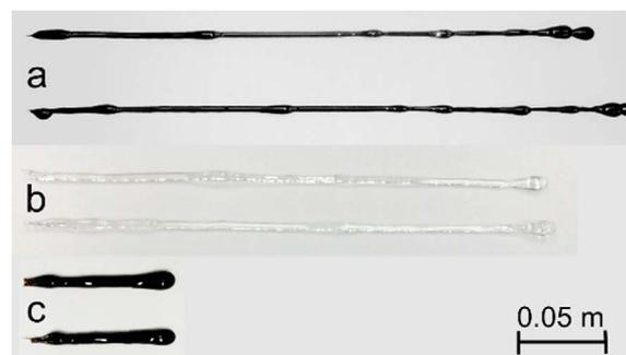
**Fig.2** - a) Droplet formation in IPT ribbons of a SG5 slag according to Tab.1 with a viscosity of  $0.079$  Pa.s at  $1300$  °C; b) IPT ribbons of a glassy solidified SG5 slag with a viscosity of  $0.139$  Pa.s at  $1300$  °C, c) IPT ribbons of a SG1 slag with a viscosity at  $1300$  °C of  $1.546$  Pa.s.
