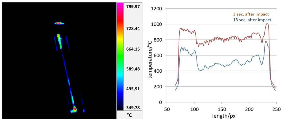
**Fig.3** - a) Thermal image of the temperature distribution of a solidifying slag ribbon and b) temperature distribution diagram of the slag ribbon, 3 and 11 seconds after slag impact.
