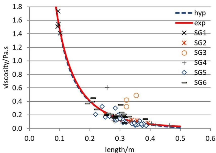
Fig.6 - Ribbon length depending on the viscosity.
