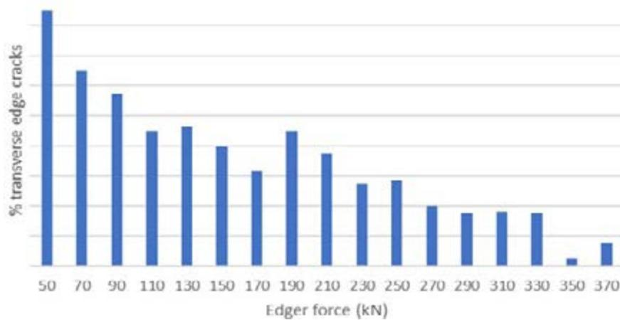
**Fig.6** - Distribution of transverse corner cracks with varying edger force. Data analysis on coils in the period from January 2017 to June 2019 clearly shows the dependence of edge crack formation on edger force.
