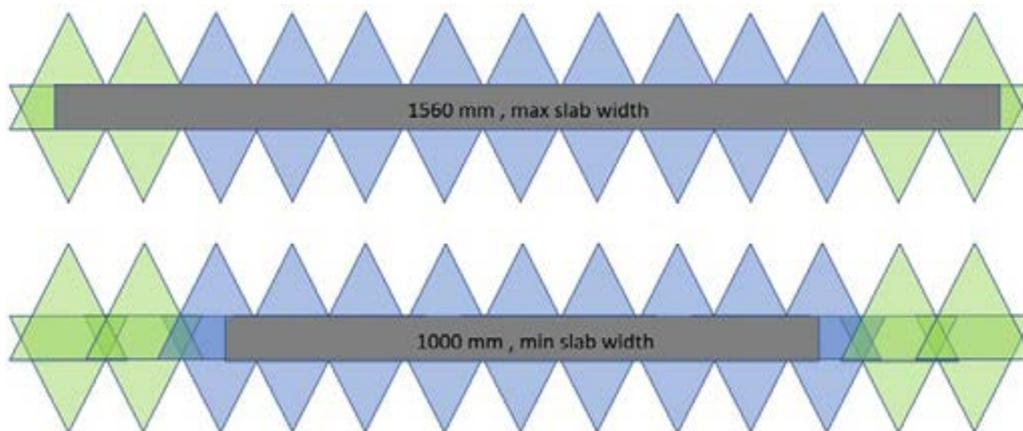
**Fig.3** - Spray nozzle configuration for narrow and broad slabs in the secondary cooling area. The outer two (in green) spray nozzles were replaced in the plant trials for spray nozzles with a 35% lower flow rate than the original nozzles.
