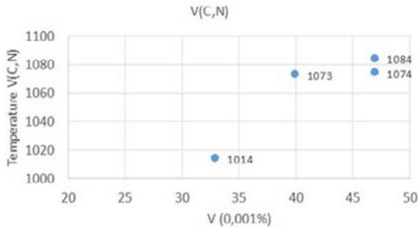
**Fig.2** - Onset of precipitation temperatures for different vanadium contents in the HSLA steel grade.
