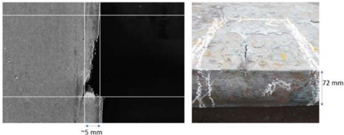
**Fig.1** - Left: Edge crack as captured by the parsytec system in the hot strip mill in the DSP.
