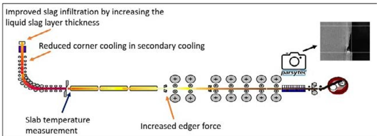
**Fig.8** - Schematics of the integrated approach for reduction of transverse corner cracks in Tata Steel's Direct Sheet Plant.
