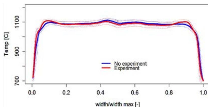
**Fig.5** - Slab temperature as measured at 16 m from meniscus. Result for low carbon steel, cast at 1450 mm slab width and at 5.7 m/min. The red line indicates the result for the trial with adapted spray nozzles and the blue line indicates the result for the original spray nozzle configuration. The dotted lines indicate the temperature at plus and minus one standard deviation.
