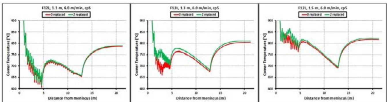
**Fig.4** - Model calculations of the temperature at the slab corners for the original spray nozzle configuration (red) and for the configuration where the outer three spray nozzles at the first secondary cooling segment were replaced by nozzles with a 35% lower water flow rate.
