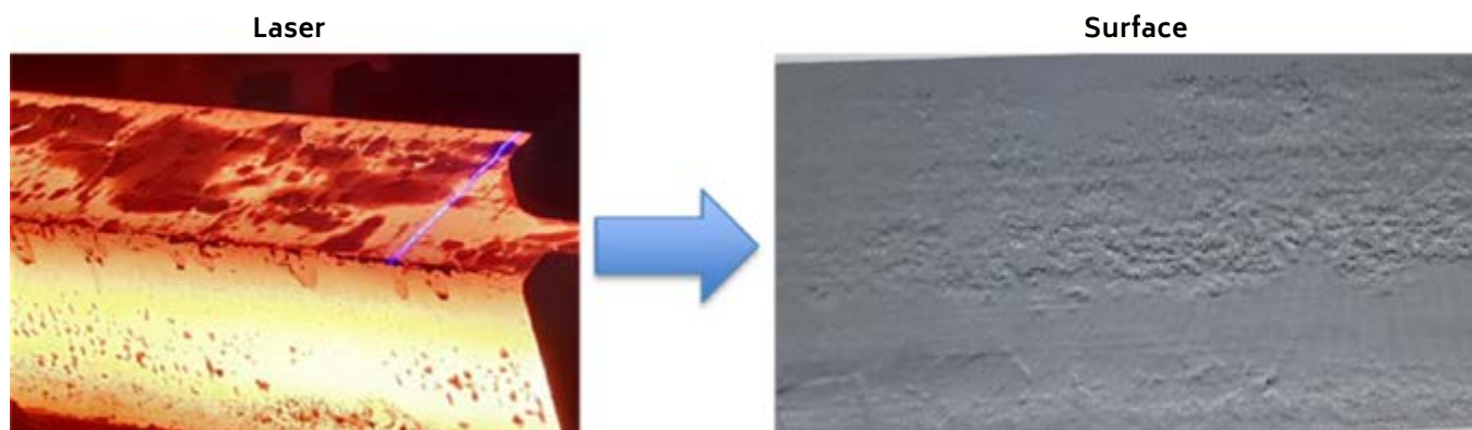
Fig.10 - On-line laser scanning and billets surface reconstruction through Deep Learning.
