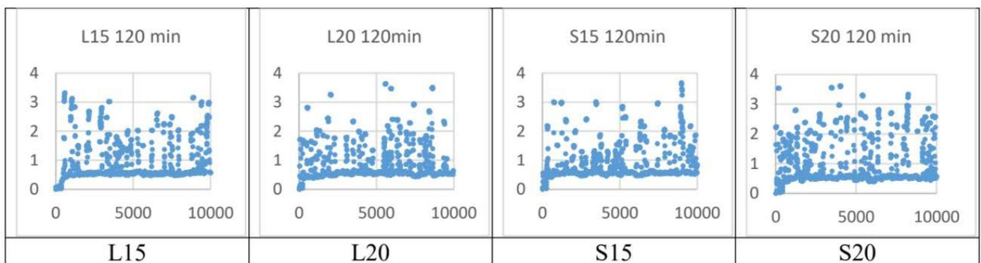
**Fig.6** - CoF as a function over time for samples L15, L20, S15 and S20 illustrating the number of adhesive events where the friction force exceeds the normal force.
