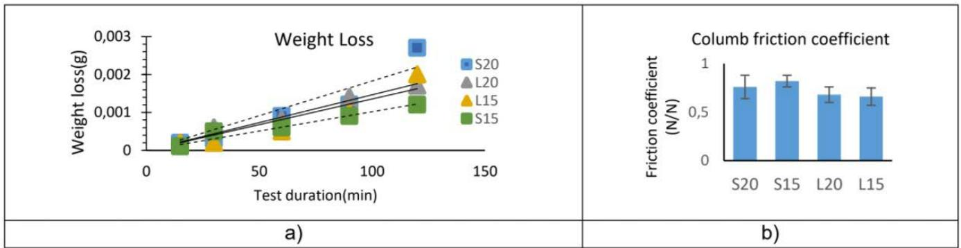
**Fig.5** - a) Mass loss from the dry sliding wear test b) CoF during the sliding wear test.
