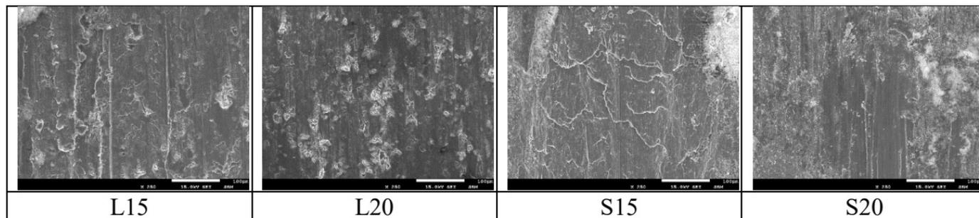
**Fig.7** - Wear surface samples L15, L20, S15 and S20 illustrating the adhesive and abrasive nature of the wear mechanisms as well as the stability of the tribo-layer. (Scale bar is 100 $\mu$ m).
