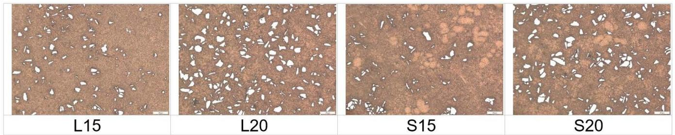
**Fig.1** - Illustration of the microstructures with L15 and L20 samples being cast using conventional high-pressure die casting and S15 and S20 being cast using rheocasting. Scale bar is 100µm.
