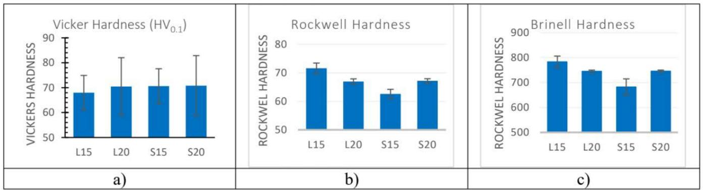
**Fig.3** - Hardness of the composite, a) Micro-Vickers results, b) Rockwell C hardness results, c) Brinell hardness converted from Rockwell hardness.
