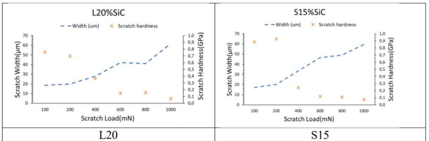
**Fig.4** - Scratch test using progressive load.
